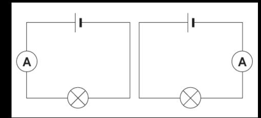
Why should an ammeter have a very low resistance? Since the entire current passes through the ammeter, It should not change the value of current flowing in the circuit.
