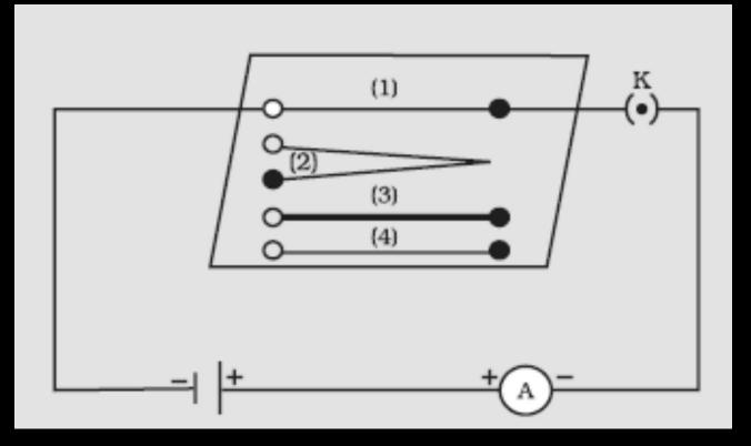
When the length of the wire is doubled, the ammeter reading decreases to one-half its initial value.
