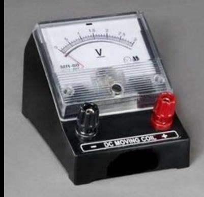
How is a voltmeter connected in a circuit? A voltmeter is always connected in parallel across the points where the potential difference is to be measured.
