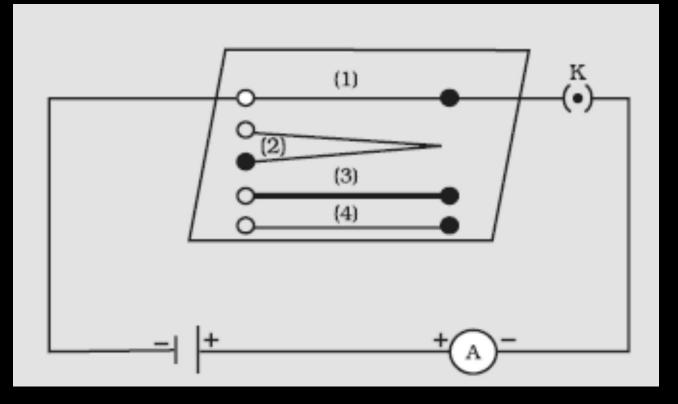
When we use copper wire of similar dimensions in place of the nichrome wire, the current in the circuit increases.
