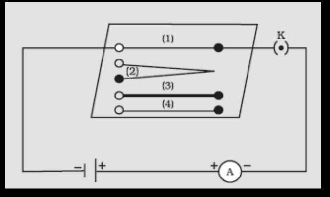
When we use a thicker wire of the same material and of the same length, the current in the circuit increases.
