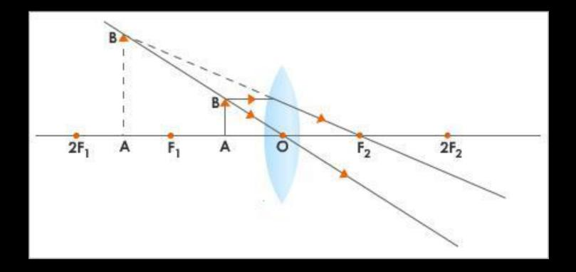
Nature: Virtual, erect, enlarged image is formed behind the lens.
