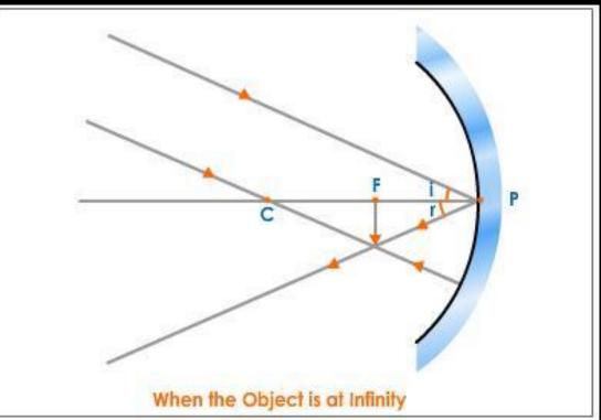
Nature: Real, inverted, highly diminished, point-sized image is formed at focus (F)
