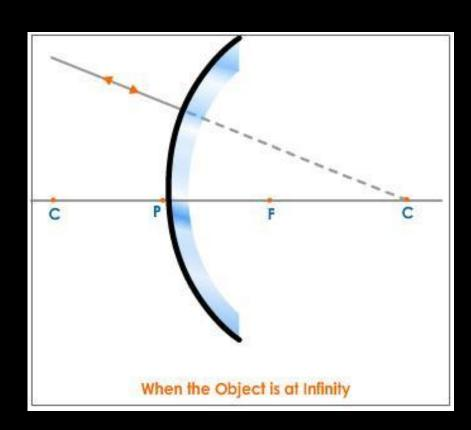
Nature: Virtual, erect, highly diminished point sized image is formed at focus F behind the mirror.
