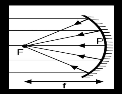
The radius of curvature of a spherical mirror is twice the focal length. R=2f
