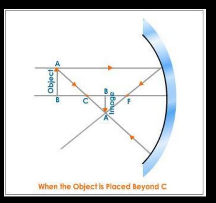
Nature: Real, inverted, diminished, image is formed between C and F
