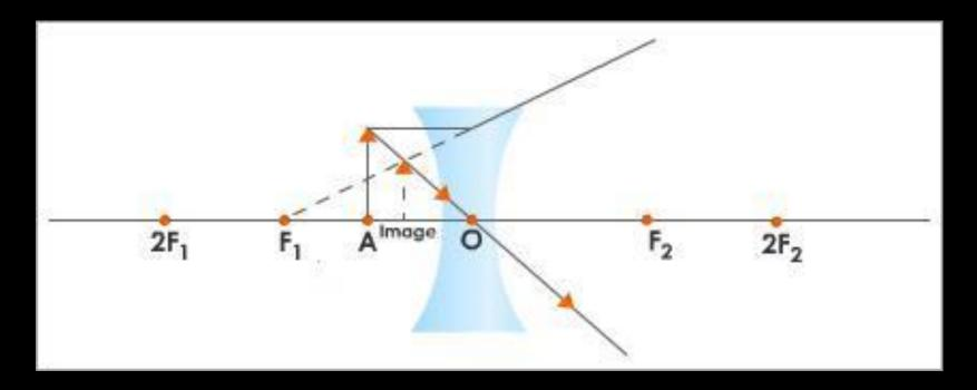
Nature: Virtual, erect, diminished image is formed between F1 and O.
