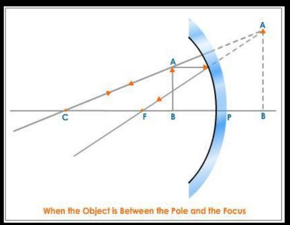
Nature: Virtual, erect, enlarged image is formed behind the mirror
