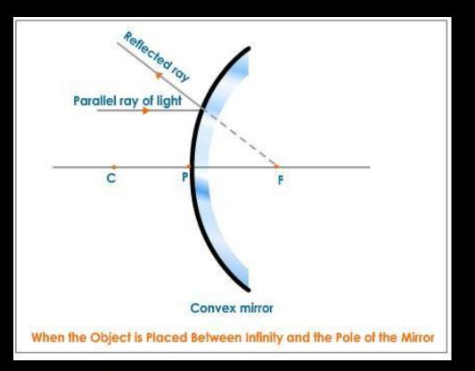
Nature: Virtual, erect, diminished image is formed between F and P behind the mirror.
