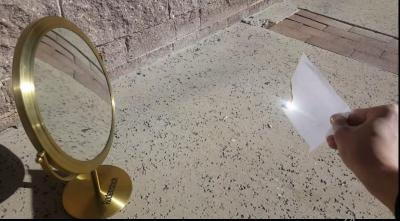
(Activity 10.2) Hold a concave mirror in your hand and direct it's reflecting surface towards the Sun. Direct the light reflected by the mirror on to a sheet of paper held close to the mirror. Move the sheet of paper back and forth gradually until you find on the paper sheet a bright, sharp spot of light.
