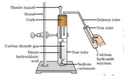
Take a spatula full of sodium carbonate in a test tube and add 2 mL of dilute ethanoic acid.
