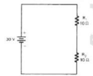
Find the current across the each resistance and total current flowing in the given circuit.
