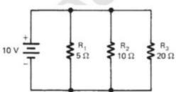
8. Find the current through 10 ohm resistor for the following circuit.
