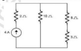
9. In the given circuit, (i) find the equivalent resistance and total current flowing in the circuit. (ii) Find the voltage and current across each resistance in the circuit.
