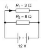
Find the voltage across each resistance in the given circuit.
