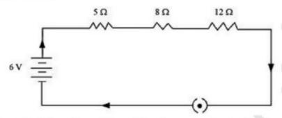
90. Redraw the circuit of Question 88, putting in an ammeter to measure the current through the resistors and a voltmeter to measure the potential difference across the 12  $\Omega$  resistor. What would be the readings in the ammeter and the voltmeter?
